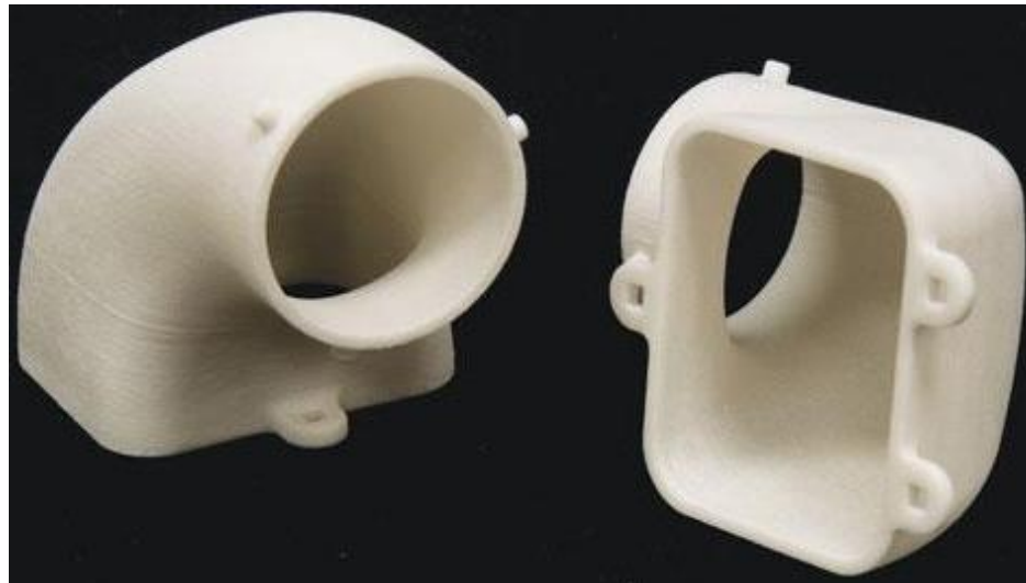
Figure 1-2: Aerospace duct made using SLS [7]
