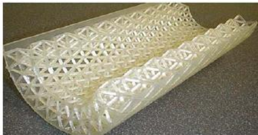
(b) Skin with 2 layers of lattice structure made using SL
